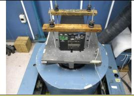
Mechanical Shock Test (±Z axis)
