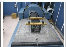
Mechanical Shock Test (±Y axis)
